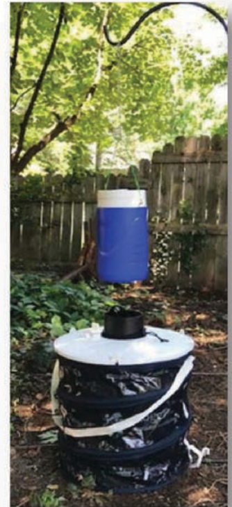
Figure 2—BG Sentinel Trap for adult host-seeking mosquitoes.
